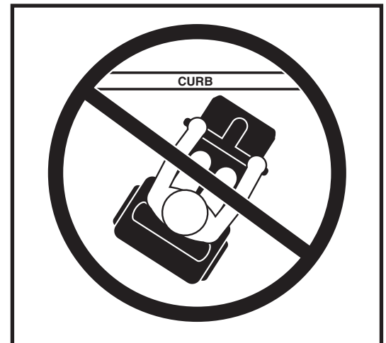
Figure 7. Incorrect Curb Approach
