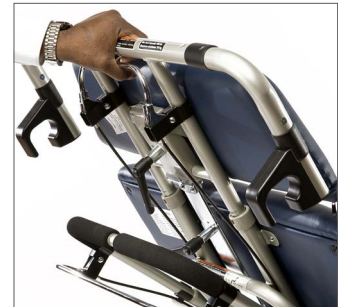
Easy to use adjustment levers allow for positioning from supine to seated position by a single caregiver.
