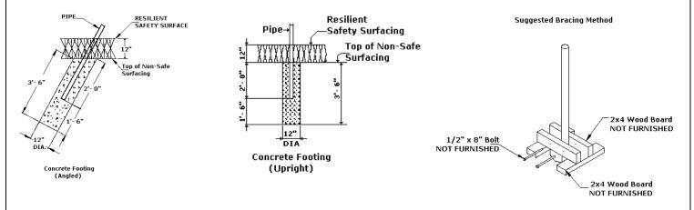
• If resilient surfacing is to be less than 12", then additional pipe should be put in concrete to maintain proper finish grade for equipment.
