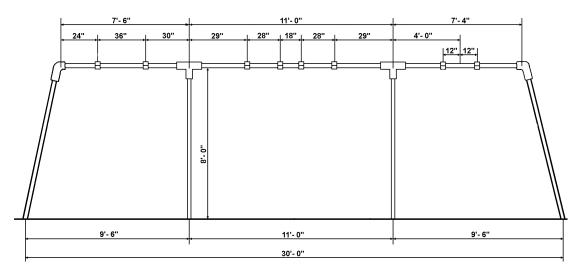
Dimensions listed are proper for components shown. Minimum spacing required is 30'' from chain to nearest support and 24'' between chairs on adjacent components measured at 5'-0'' above the resilient surfacing.
