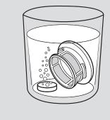
After cleaning it, replace the filter cap in the filter cap in the filter cleaning it, replace the filter cap in the fil to the **b** position
