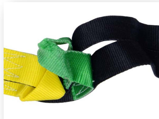
Stiffened and Brittle Loop Strap
