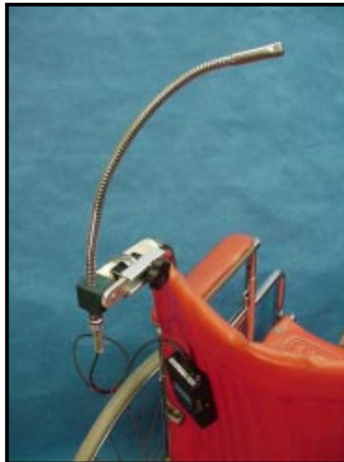
Quick Release Mount attached to wheelchair cane handle (Two Views).
