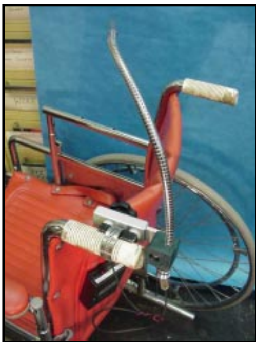
Quick Release Mount attached to wheelchair cane handle (Two Views).
