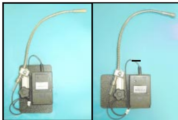
(a) Vertical mounting (b) Horizontal mounting Gooseneck attached to mounting plate with split block clamp. SCATIR switch attached to mounting plate beside gooseneck.
