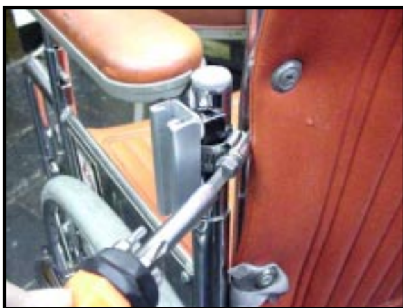
Quick Release Mount attached to wheelchair arm rest tube.
