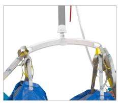
Place the straps from the lifting sling on the hooks on the carry bar. Start with the shoulder straps (from the back) and then place the loops of the leg straps on the hooks of the carry bar.
