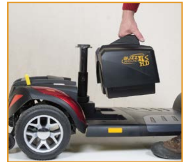
Step 2: Pull out the battery pack!
