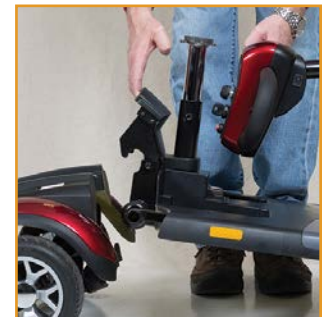
Step 4: Pull forward on the drivetrain release lever to separate the front and rear frame sections!
