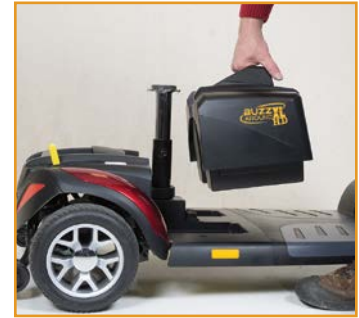
Step 2: Pull out the battery pack!
