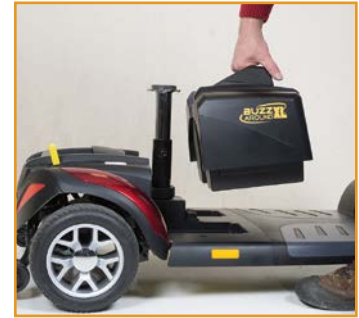
Step 2: Pull out the battery pack!
