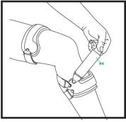
4. Tighten the outer straps (#4) to the upper and lower end of the metal bar. Following the blue line, trim the excess velcro off if the strap is too long.
