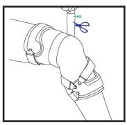
5. Tighten the straps (#5) to the upper of the metalbar. Following the blue line, trim the excess velcro off if the strap is too long.
