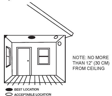
Figure 5: RECOMMENDED SMOKE ALARM MOUNTING LOCATIONS.
