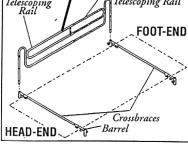
WARNING: To prevent damage to levers and motors of articulating beds, make certain that when the foot and head-ends are raised that the telescoping length of the bed rail is not less than 47 inches. Otherwise the bed rail has bottomed-out and will bind the drive mechanism of the bed. Fither the bed rail or the bed will be damaged.
