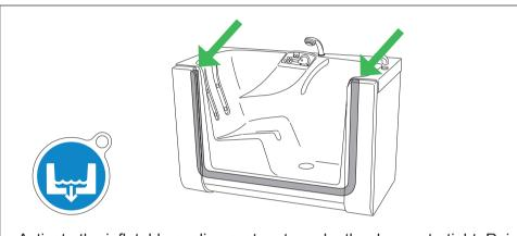
Activate the inflatable sealing system to make the door watertight. Raise the door and press the door seal/drain button.
