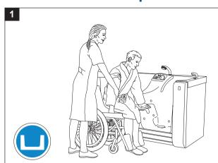
Press the door down button to lower the door to its lowest position.
