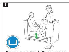
Press the door down button to lower the door to the lowest position.
