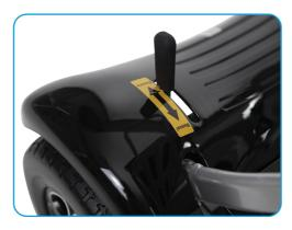
**NOTE:** When in Manual, the scooter braking system is disengaged. Power can be turned on in manual mode, but the control system will automatically cut off the motorized functionality of the scooter.
