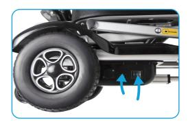
Assemble the power block and power cord. Connect the power block to the scooter, and plug into a standard wall outlet.
