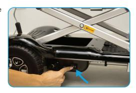
4. With the scooter unfolded, connect the battery to the designated battery port.
