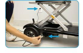
not charge the scooter) or you can plug it directly into the top of the battery itself to charge the scooter battery.
