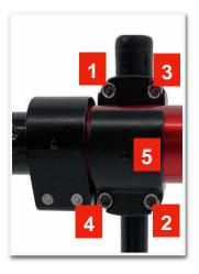
(Tighten down the screws in a diagonal configuration #1-4, **do not over tighten the screws to avoid damaging them.** Finish w/ the set screw last #5.)
