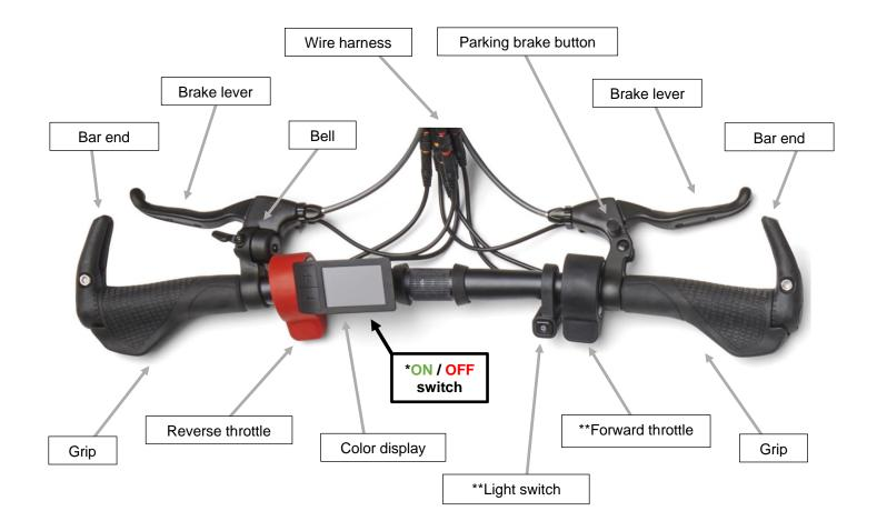
**\*To turn on the Firefly**<sup>™</sup>**2.5**: press the power switch on top of the battery until the battery's LED light display turns on. Then press and hold the color display power switch for 3~5 seconds. When you see the Rio mobility logo - the unit is now powered up.
