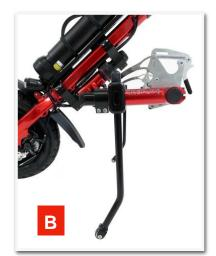
Push the kickstand clamp up against the coupler clamp "**C**". Tighten the screws loosely at first using your 4mm hex wrench. Fully tighten down the screws in a diagonal configuration. If the clamp pulls too close on one side, back off that screw and cinch down the remaining screws with more tension.
