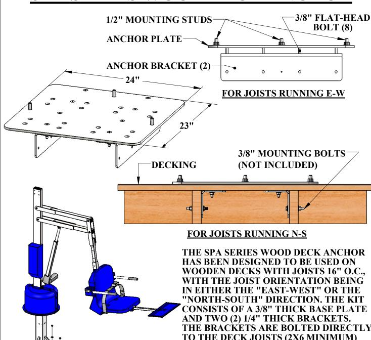
WOODEN DECKS WITH JOISTS 16" O.C., WITH THE JOIST ORIENTATION BEING **CONSISTS OF A 3/8" THICK BASE PLATE** THE BRACKETS ARE BOLTED DIRECTLY TO THE DECK JOISTS (2X6 MINIMUM) AND THE ANCHOR PLATE BOLTS THRU THE DECKING TO THE BRACKETS. THE KIT COMES WITH EIGHT (8) FLAT-HEAD BOLTS FOR ATTACHING THE BRACKETS. ALL MATERIALS ARE STAINLESS STEEL. AND POWDER COATED FOR LONG LIFE. THE WOOD DECK ANCHOR IS FOR THE SPA LIFT ELITE AND SPA LIFT ULTRA.
