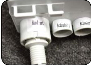
NOT Properly Inserted: The cord plug is flush with or sticking out of the outlet
