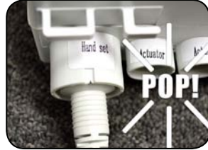
Properly Inserted: The cord plug is recessed into the outlet
