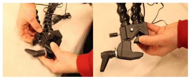
2. You can also remove one of the Easy Flex Dual Ultimate Switches from the clamp if only one switch is needed. To do this loosen the set knob on the clamp, then depress the spring loaded pin and lift up on the Flex arm to remove the switch from the clamp. See photos below.
