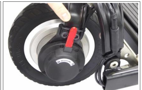
12 Check that the magnetic brake is in the LOCKED position to engage the motor.
