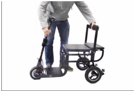
8 ...the scooter will lock itself into its open position.
