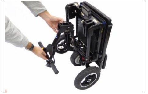
3 Pull the handlebars out and upward...
