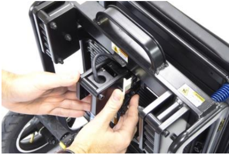
1 Release steering column latch...
