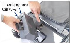
Remove the battery by unlocking using the key and applying gentle pressure. The battery has points for charging and for powering a mobile device.
