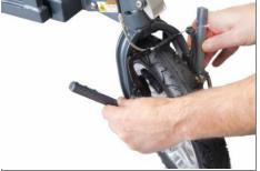
....and make sure the column key **locks** into place under latch 'A'.
