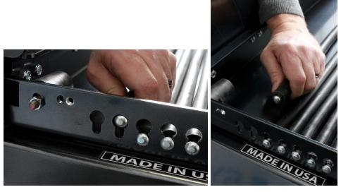
3) To completely remove elasticord move to the headend of the machine and loosen the rod holding the loop end of the elastic in place.
