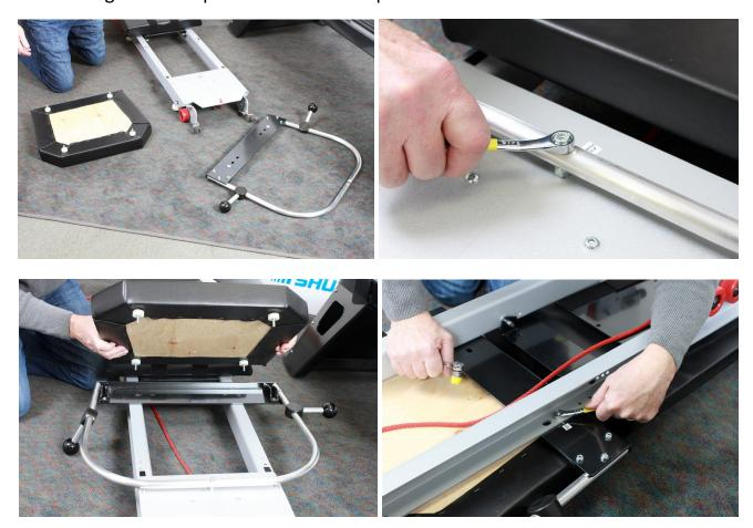
14) Place the seat on the carriage matching the 13 & 14. Remove the 4 nuts and washers from under the seat and secure the seat to the carriage rails through the handle bar and through the matching holes on the carriage.
