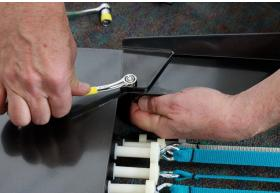
7) Place the *Head End Stand* on the *Rails* aligning the number 3 & 4. *The* four bolts and nuts must be removed and reinstalled through the four appropriate holes. Lightly tighten bolts to be tightened in next step.
