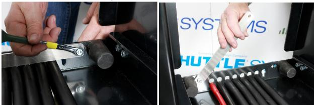
2) Once the bracket has been loosened elasticords can be removed from the slotted plate.
