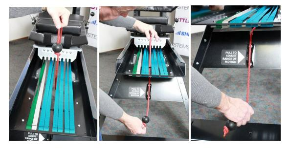
22) Place the red Range of Motion Control Rope with the round ball on end in the black plastic clam cleat rope lock located at the head end stand. This rope is used to adjust the start point of the carriage travel and provides a soft stop at the foot end of the travel. 23) Reinstall the two black rubber carriage travel limiter stops at the end of the rail.
