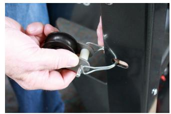
**5)** Unravel the pulley ropes and secure the free end of the pulley ropes to the black plastic clam cleat rope locks at each rear edge of the seat pad.
