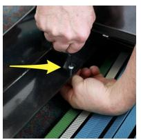
8) Place the *headend stand base plate* with the rubber feet onto the the stand structure with the feet pointing up and match the 5 & 6. Tighten all nuts on the *Wings* and *Stand*.
