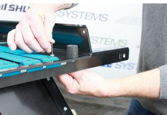
3) Secure with the two bolts and nuts in the same orientation as received.
