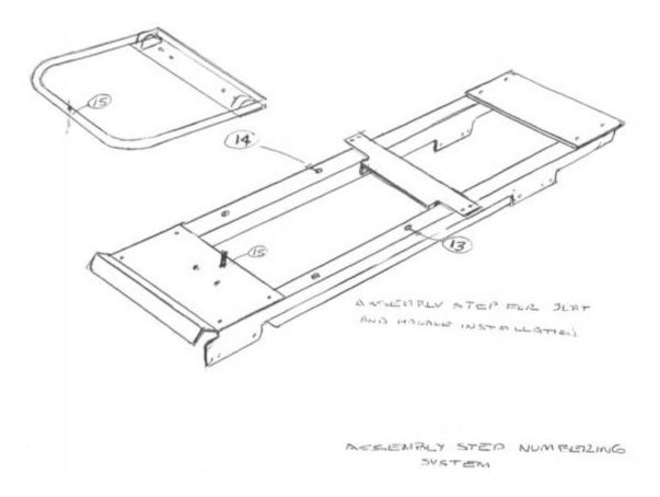
**15)** The hole in the front center of the curved handle structure should be placed over the bolt on the foot rest. Add the nut, tighten, then add black nut cover.
