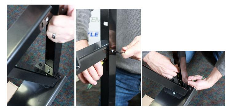
**4)** Matching the 11 & 12 with the stand base. Secure the towers with the crossbar and the base plate with the bolts and nuts provided.
