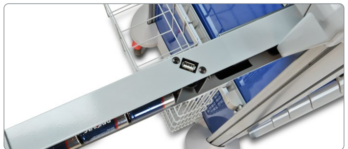
Slideout USB port for field software updates for onboard electronics.
