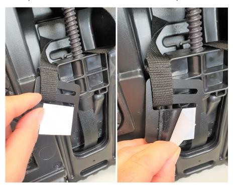
Position metal locking plate as far as possible to the front of slot. Then press down metal locking plate so adhesive surface will glue to seat shell.
