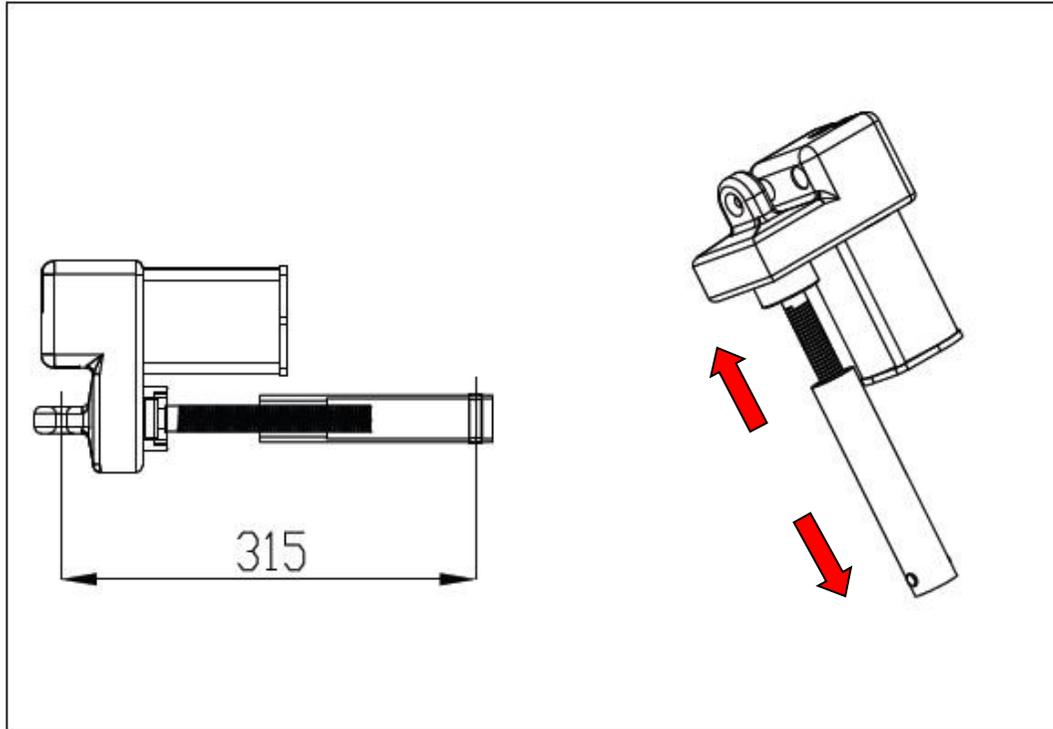
**Incline Range must be adjusted to 315 mm minimum prior to installation.**
