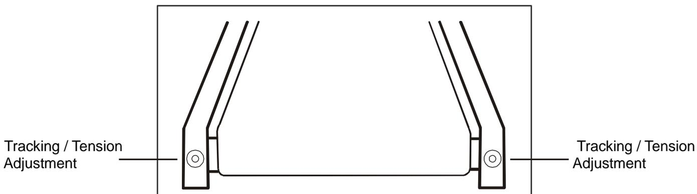
**Note:** Adjustment is through small hole in the end cap.
