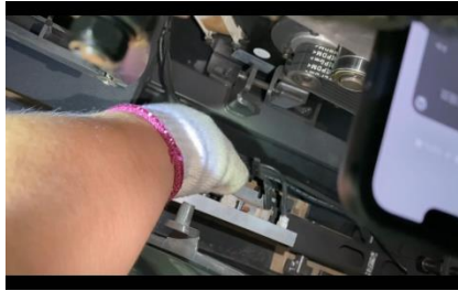
2. Remove the connection wire of control board
