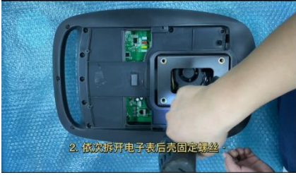
1 Remove the rear cover of console
