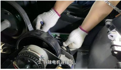
5. Remove the connection wire of control board
