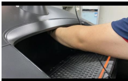
2. Cut off the fixed tie at the bottom of upright frame
