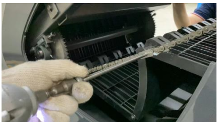
Pull out the pedal fixing shaft from one side
