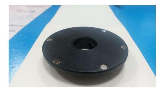
3. Check sensor head – the internal sensor should be no more than a few millimeters inside the hole.
