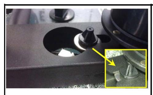
Install the Speed Sensor as shown.
