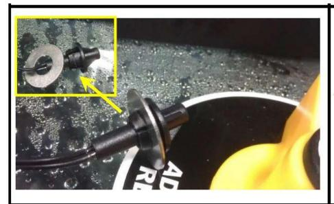
Remove the washer from the Speed Sensor
