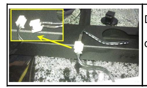
Disconnect the sensor cables
