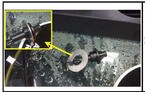
Fit washer onto the new Sensor
