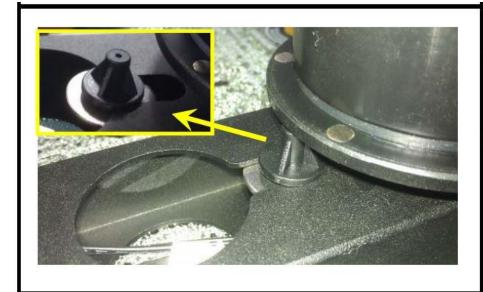
Pull the Speed Sensor out of the frame
