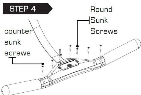
Reinstall the 6x M3x20mm Counter Sunk Screws and 2x M3x12mm Round Sunk Screws.
