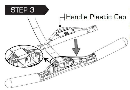
Belt is placed in the fixing slot and covered Handle Plastic Cap as shown in picture.
