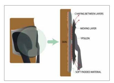
Laboratory tests reported 0.36 coefficient of friction between the two gliding fabrics which would relieve the amount of pressure against the tibia by approximately 25%.
