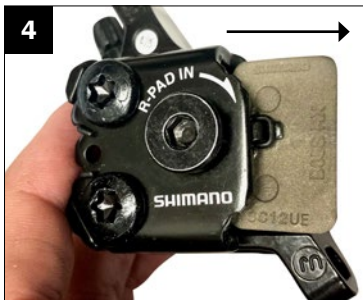
4. To remove pads, push pads through caliper.
