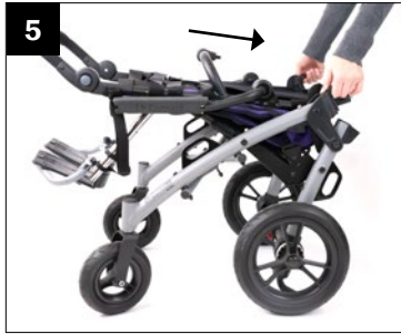
5. Grasp each side of the frame and pull up on the Base Frame Trigger Lock and then pull back towards yourself to collapse the chair.
