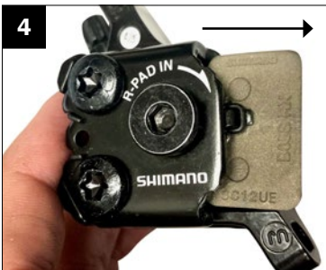
4. To remove pads, push pads through caliper.
