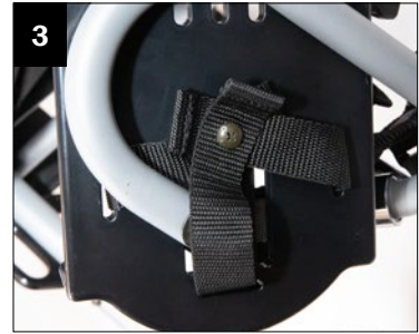
3. Bolt strap to underside of footplate using a phillips screwdriver.
