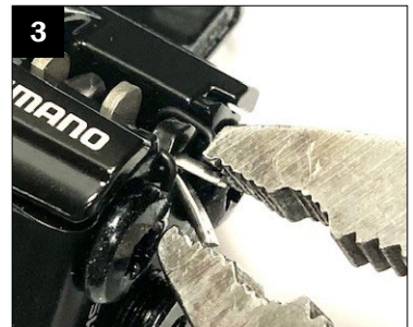
3. Remove cotter pin with pliers.
