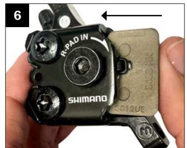
6. Reinsert pads into caliper. Follow steps 3-1 in reverse
