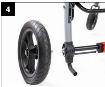
4. Align axle to wheel lock bar.
