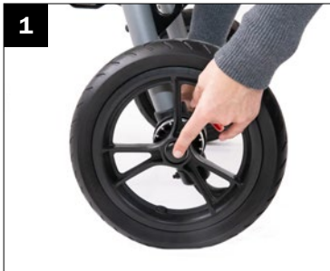
1. To remove, press down and hold the center wheel cap.
