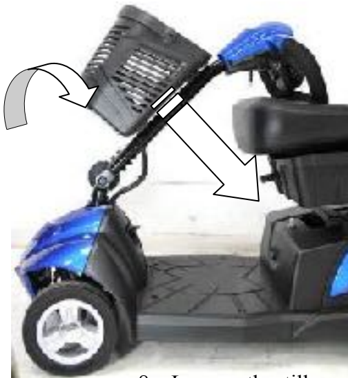
8. Loosen the tiller adjustment knob and fold down the tiller and retighten knob.
