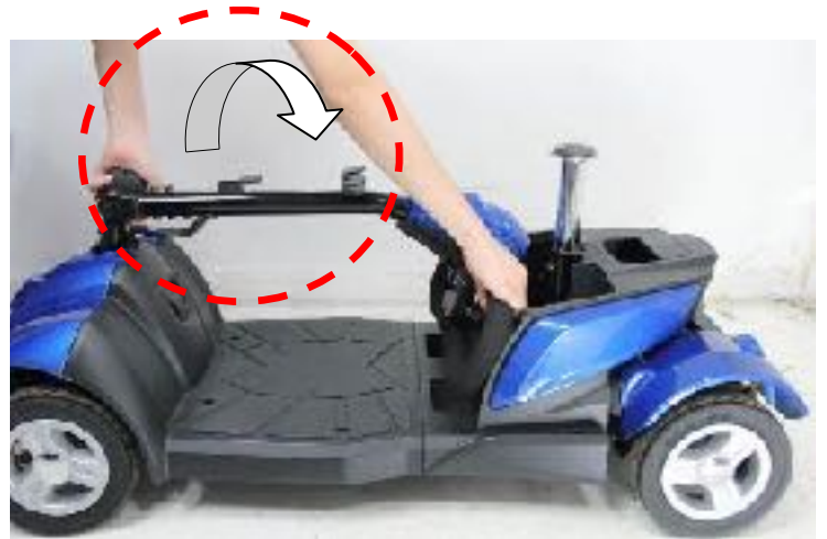
8. Loosen the tiller adjustment knob and fold down the tiller and retighten knob.
