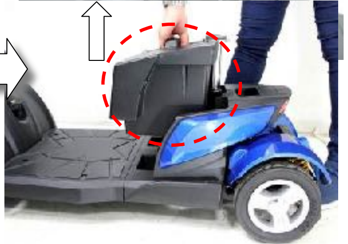
7. Pick up the battery pack and remove it from the scooter.
