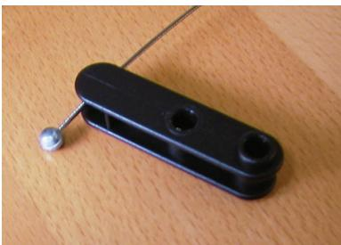
**Replace the brake cable. The ball at the end of the cable will seat in the rocker housing.**
