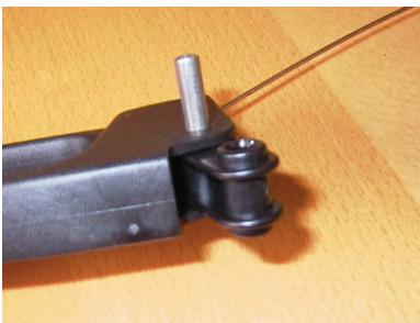
**Use a small tool or the screw from step one to push the rod out of the cable housing**
