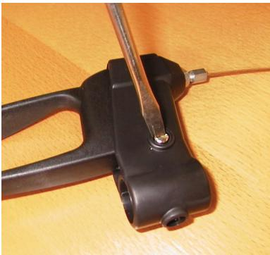
**Open the screws on the side of the brake handle, using a flat blade screwdriver. Notice that one side is a hex shape and will not turn freely, unscrew from other side.**
