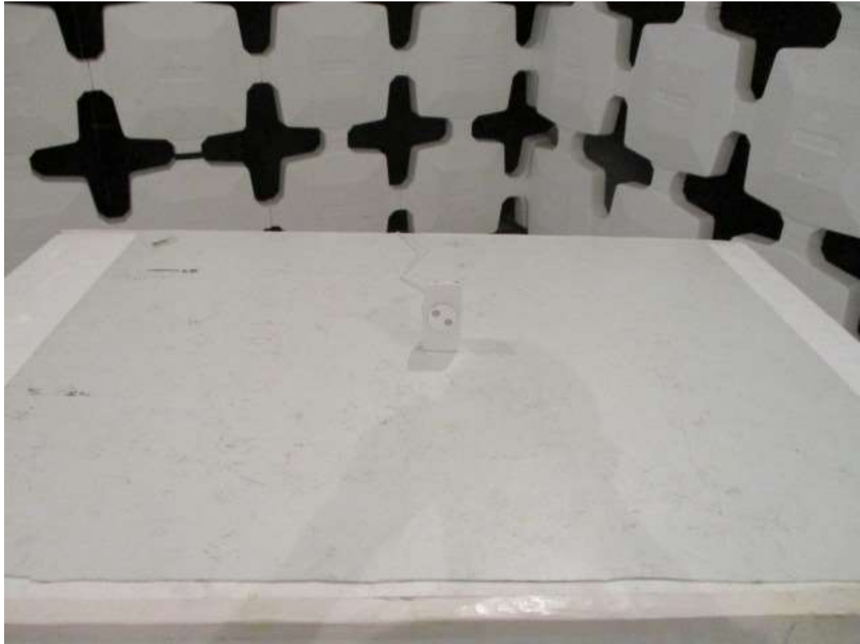
Figure 8. Radiated Emissions Test Setup Photo, Close-up
