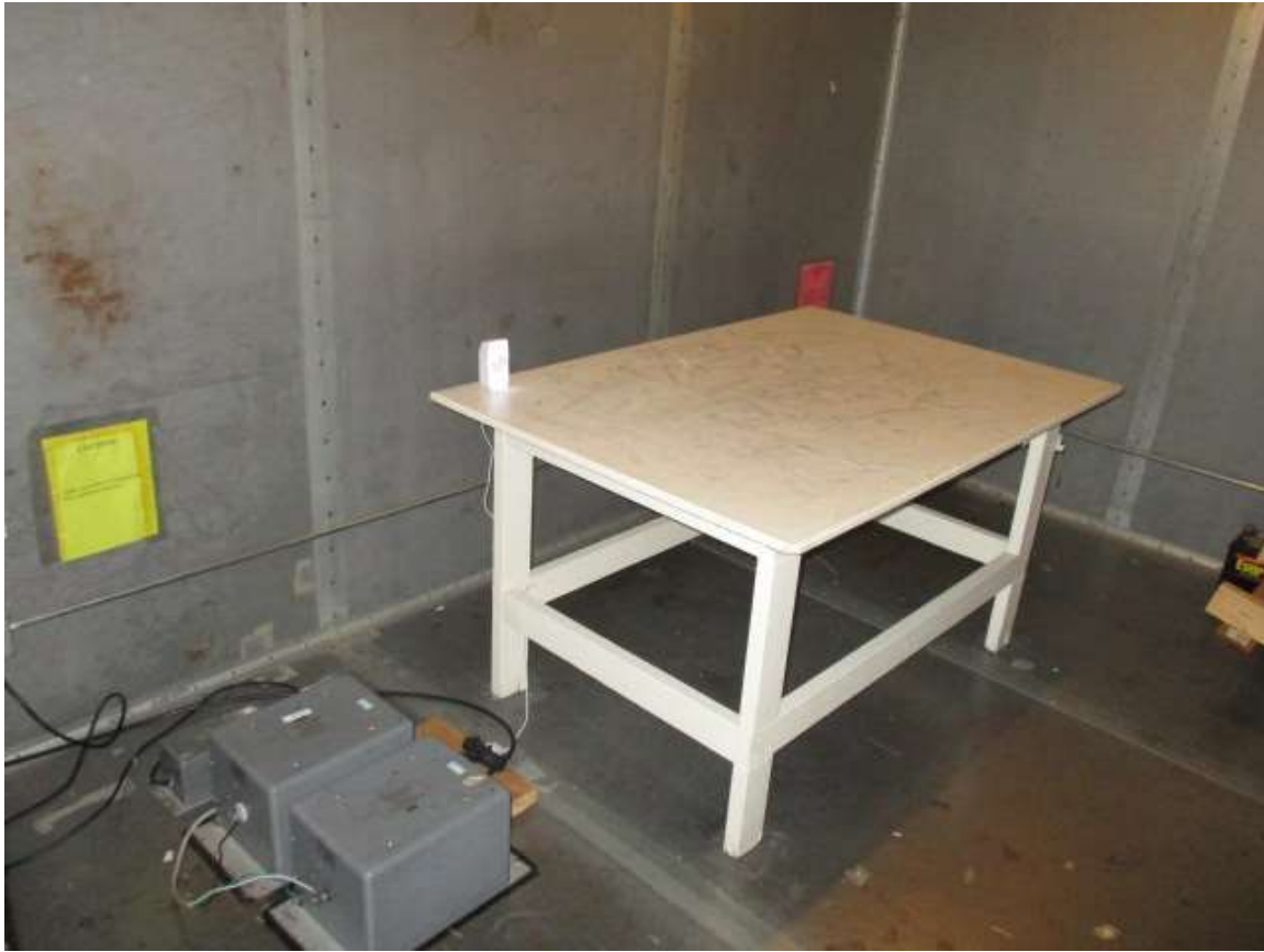
Figure 12. Conducted Emissions Test Setup Photo
