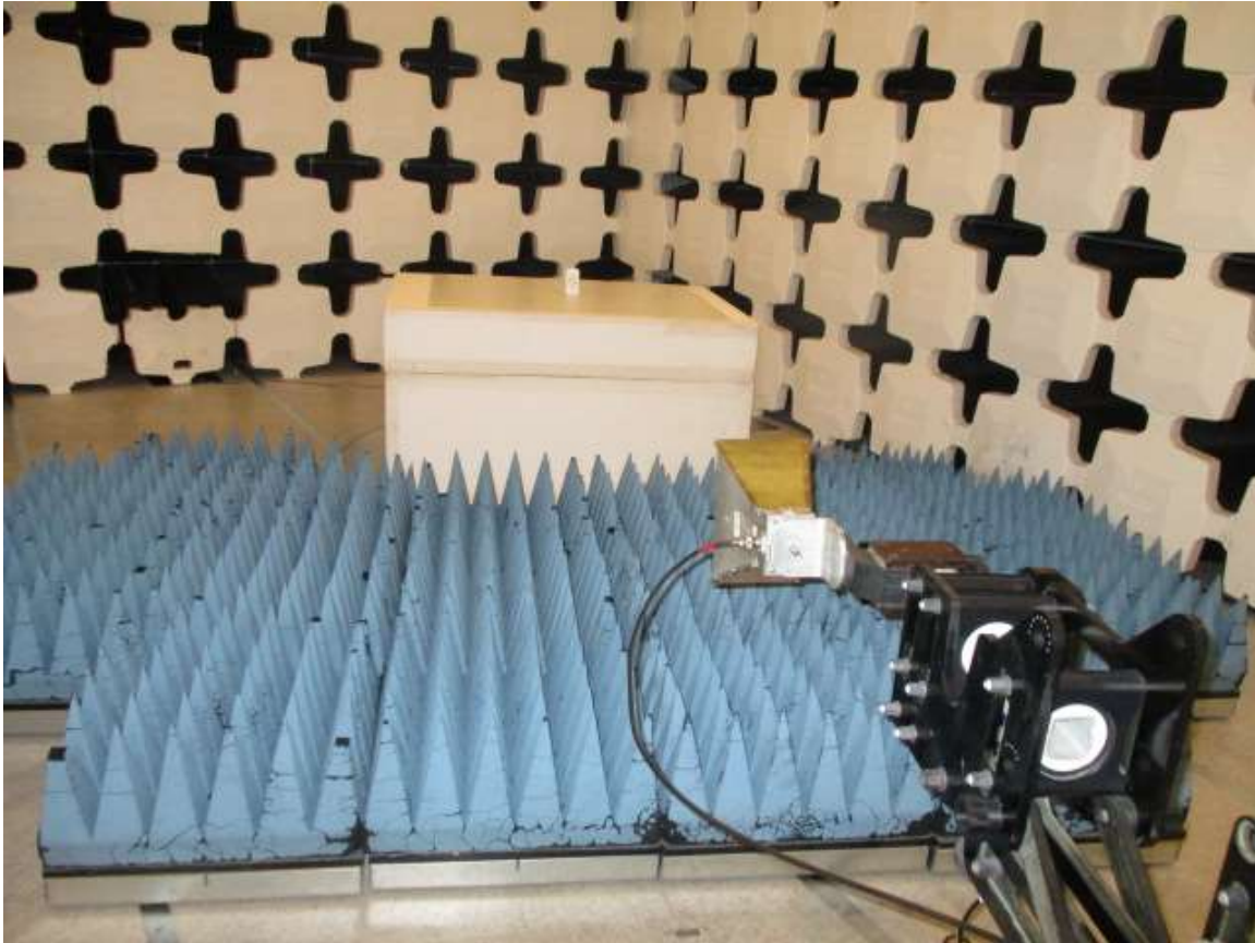
Figure 11. Radiated Emissions Test Setup Photo, above 1 GHz
