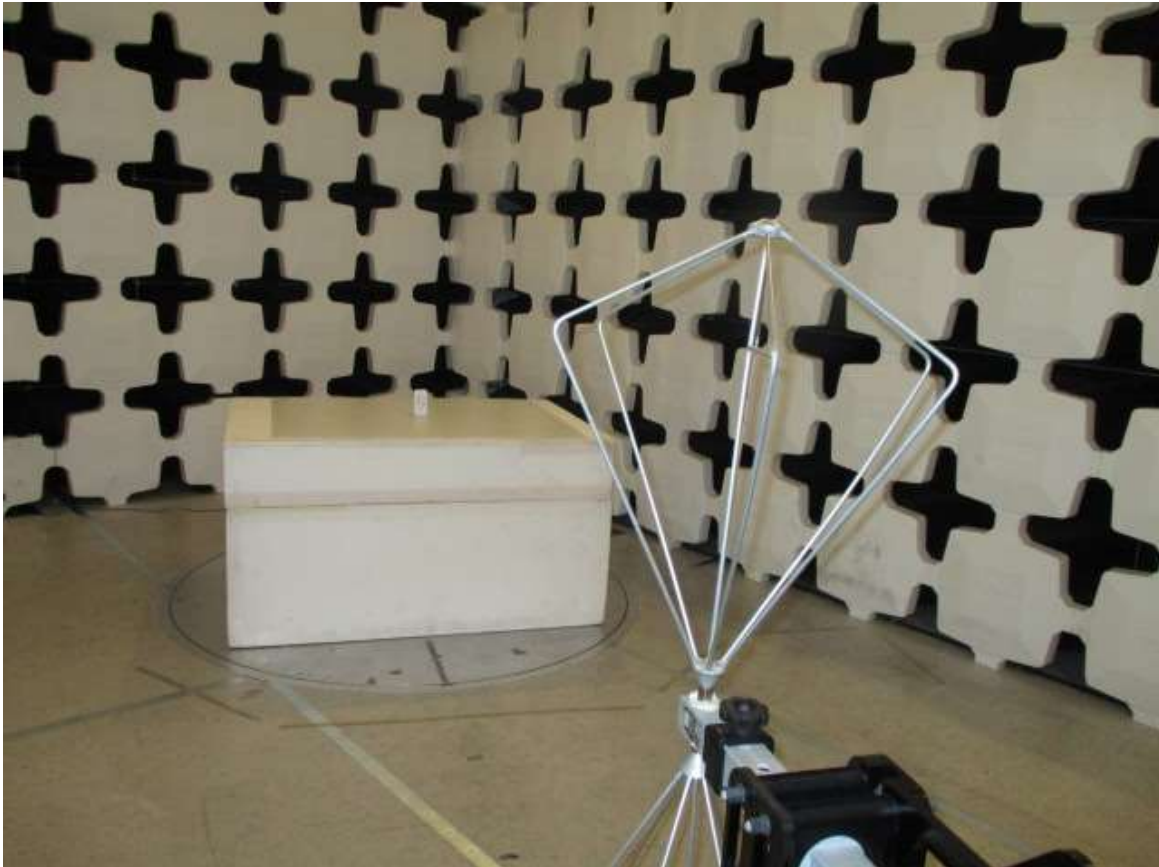
Figure 9. Radiated Emissions Test Setup Photo, 30 – 200 MHz
