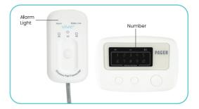
3. The pager will beep to signal a successful connection. The pager will then re-enter programming mode so that you can connect other devices. If you do not need to connect other devices, press and hold both the UP and DOWN buttons for more than 5 seconds to exit programming mode.
