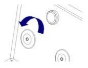
Rotate the jet cover anti- clock-wise until it can be removed easily.
