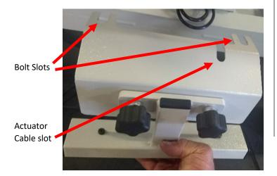
Align the actuator connector cable and the bolts into the specified slots and slip the bracket into place.
