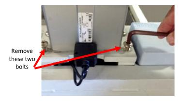
Position the AutoStep attachment bracket behind the bolts. Notice two slots for the bolts, and one slot for the actuator cabling.
