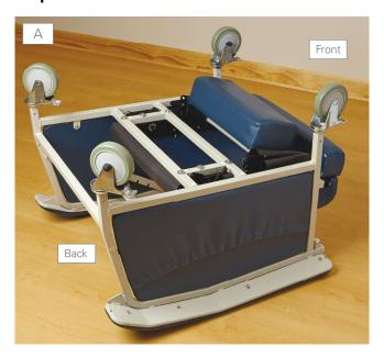
A. Turn the chair base upside down and attach the casters to the legs of the chair base. The swivel locking casters should be placed on back legs of the chair base and secured with the nuts, bolts and caps provided. The front of the chair receives the directional non swivel locking casters.
