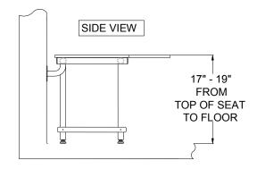
Place the seat in an upright position with the mounting flanges placed firmly against the shower wall.
