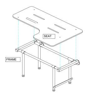
Mount the seat top to the frame in the desired configuration.
