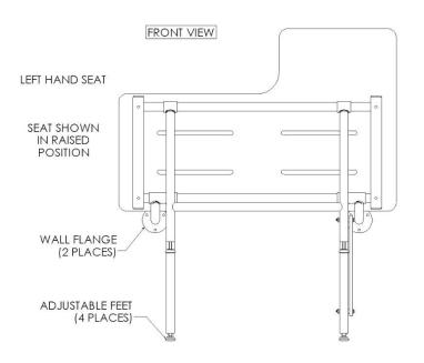
Level the seat by changing the adjustable rubber feet to the desired mounting height (17"-19"). Tighten the lock nuts.
