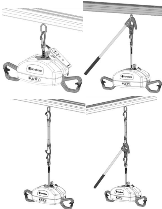
Figure 8: Top Left – Standard Connection. Top Right – Reacher Arm Connection. Bottom Left – Lanyard Connection. Bottom Right – Reacher arm and Lanyard Connection.
