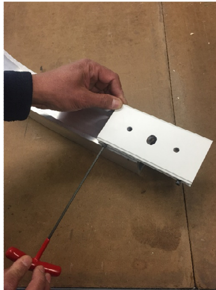
Figure 15 – Tighten with 3mm T-Handle
