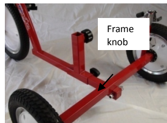
Main and rear frames attached
