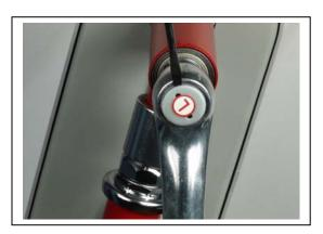
2) Use a 14 mm Socket and Ratchet and turn the crank arm securing bolt counter clockwise until crank arm securing bolt is completely removed.
