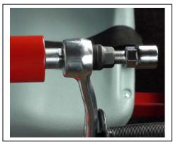
5) Using either a 16 mm wrench or adjustable wrench turn the forcing screw clockwise until the crank arm slides off the shaft.
