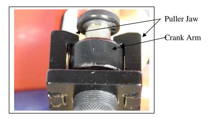
4) Use either a 16 mm or adjustable wrench and turn the forcing screw clockwise until the crank arm slides off of the shaft.
