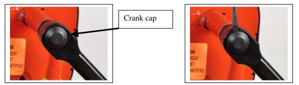
2) Use the 6 mm Allen Wrench and insert it into the Allen Bolt and turn counter clockwise until crank arm securing bolt is completely removed.
