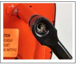
3) Slide crank removal tool over crank arm making sure that puller jaw is behind crank arm.
