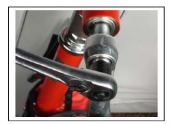
3) Remove the crank adaptor from the puller jaw by turning it counter clockwise. *Note: The puller jaw is not used on the AM-12 or AM-16 crank arm removal.*
