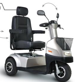
All operational controls including lights, horn and battery display are conveniently located in the center of the one-hand operation Delta handlebar
