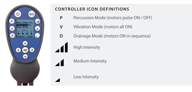
□ AffloVest will start in the medium intensity mode by default. Pressing the following buttons will update the treatment whether AffloVest is running or not:
