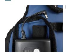
Open battery compartment and disconnect battery as shown.
