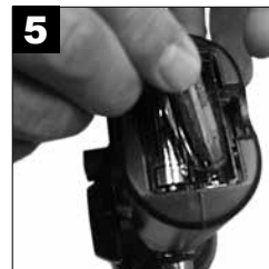
Install batteries if necessary (observe polarity).
