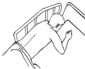
Entrapment between the bed rail and mattress
