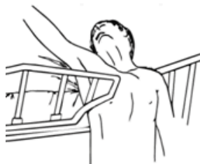
Entrapment between split bed rails
