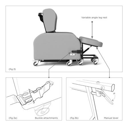
Before changing the angle of leg rest, the User or Patient must ensure there are no objects in the immediate environment that could obstruct the leg rest elevation or come into contact with the Patient's legs. Using the manual lever located under the front of the leg rest, move the leg rest until it is in the required position and release the lever. (fig.3b)
