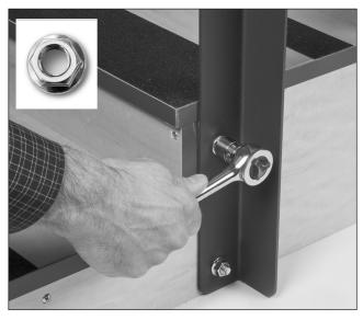
Position wooden handrail so holes in handrail line up with holes in steel uprights. Insert the 1-1/4" Phillips head bolts with a 7/8" washer through patient side of the handrail and then through the uprights on the opposite side. Finger tighten with the 7/16" washer nuts. Repeat for opposite side.
