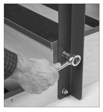
FOR SAFETY PURPOSES, TAKE TIME TO CHECK ALL BOLTS AND NUTS TO INSURE THAT THEY ARE SECURELY TIGHTENED AND THAT THE EQUIPMENT HAS BEEN PROPERLY ASSEMBLED ACCORDING TO THESE INSTRUCTIONS. CLEAN ACCORDING TO YOUR FACILITY'S STANDARDS BEFORE USE.
